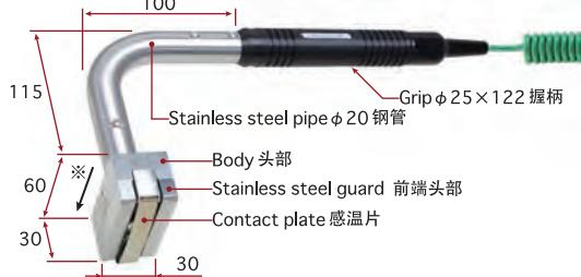
※ Direction of movement (from right side) 滑行方向(右) (mm)
